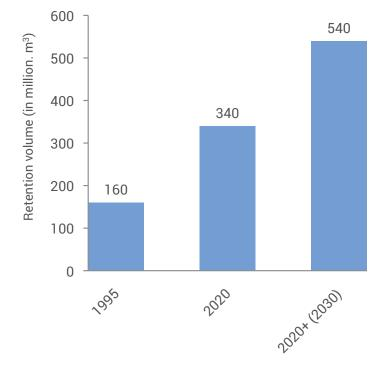
The figure shows retention volumes for different development states of the Rhine, especially in 2020 (around 340 million m³) and 2030 (planning, 540 million m³).
