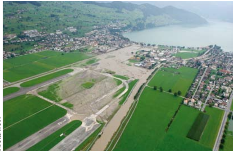
In order to protect the place of Buochs (CH) on Lake Lucerne against floods, the Engelberger Aa is, in the event of floods, led across the airport.
