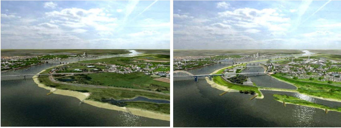
Figure 5b: Example of a river extension measure at Lent/Nijmegen, Netherlands. Dike relocation Lent, left: present situation, right: future situation (Programme "Room for the River", project "Room for the R. Waal" http://www.ruimtevoordewaal.nl /©: Ruimte voor de Waal.)
